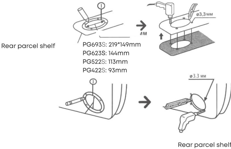
2. Cut out opening and drill holes. Make sure that the speaker is secured in such a way that it cannot slip or slide. Use the screws provided for this purpose.
